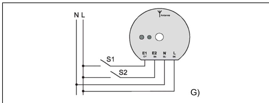
the universal transmitter transmits switch-on telegrams when closed and switch-off telegrams when opened (see fig. G).
