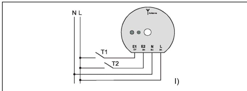
For operation of one radio-control dimming actuator.
