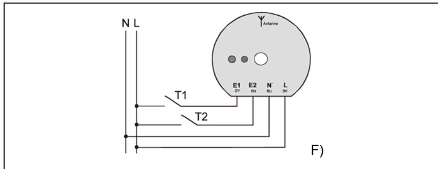
For independent control of two radio-control dimming actuators.
