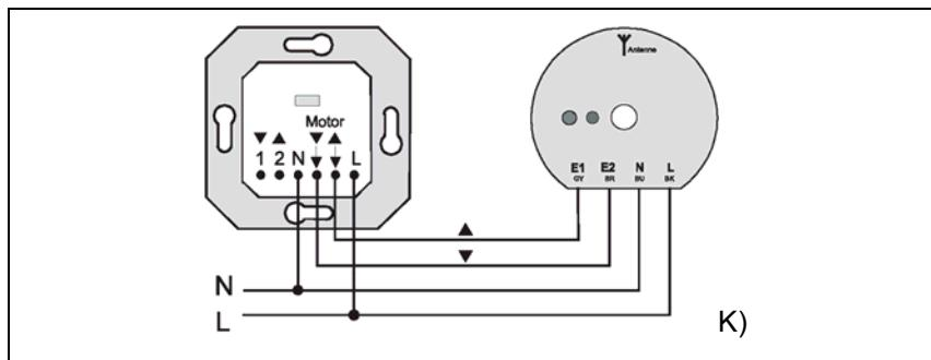
For controlling of a radio-control blind/shutter actuator.
