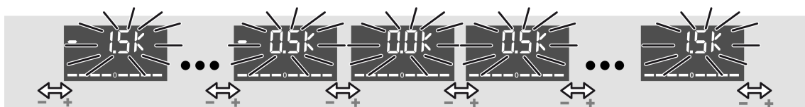
Figure 16: Setting the setpoint shift
