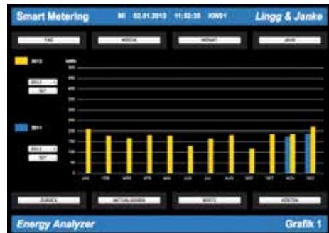
For the graphical presentation and evaluation of the metering data the network coupler "graphic" is needed. The consumption data can be displayed convenient via computer or smartphone.
