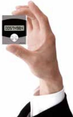
The optical sensor takes a picture of the counter every minute. This recorded meter reading gets translated via an identification algorithm to digital data.
