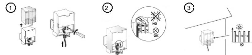
Polarity of the antenna connection is to be observed!
