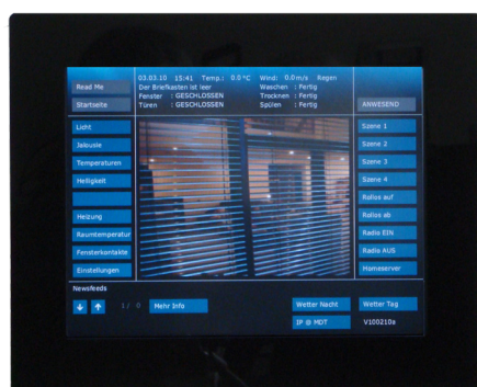
Fig.: 10,4" VisuControl Touch Panel
