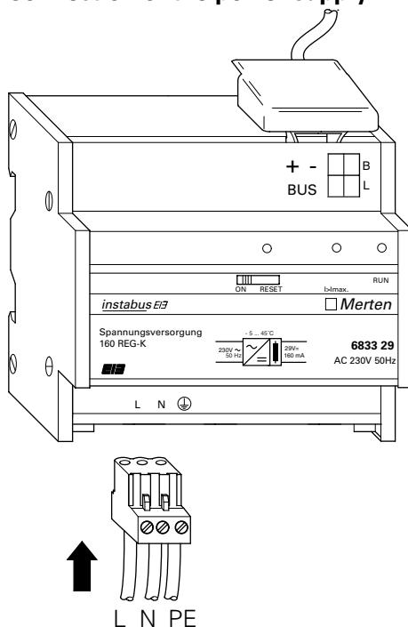
The mains voltage connection is carried out via plug-in terminals with screw connection. The cables can be screwed onto the plug-in terminal before installing the device and then inserted at a later date.
