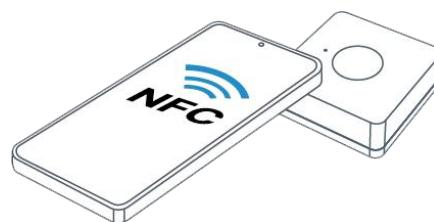
5. Basic information and settings of devices will be shown on ToolBox if it's recognized successfully. You can read and configure the device by tapping the Read/Write button on the App. In order to protect the security of devices, password validation is required when first configuration. The default password is **123456**.
