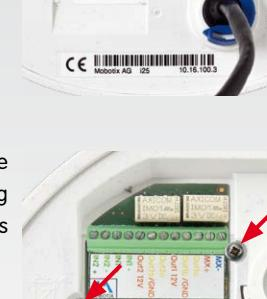
In order to release the back cover, **cautiously** press upward as indicated by the blue arrow. If you are using a flat-head screwdriver, simply turn the screwdriver.
