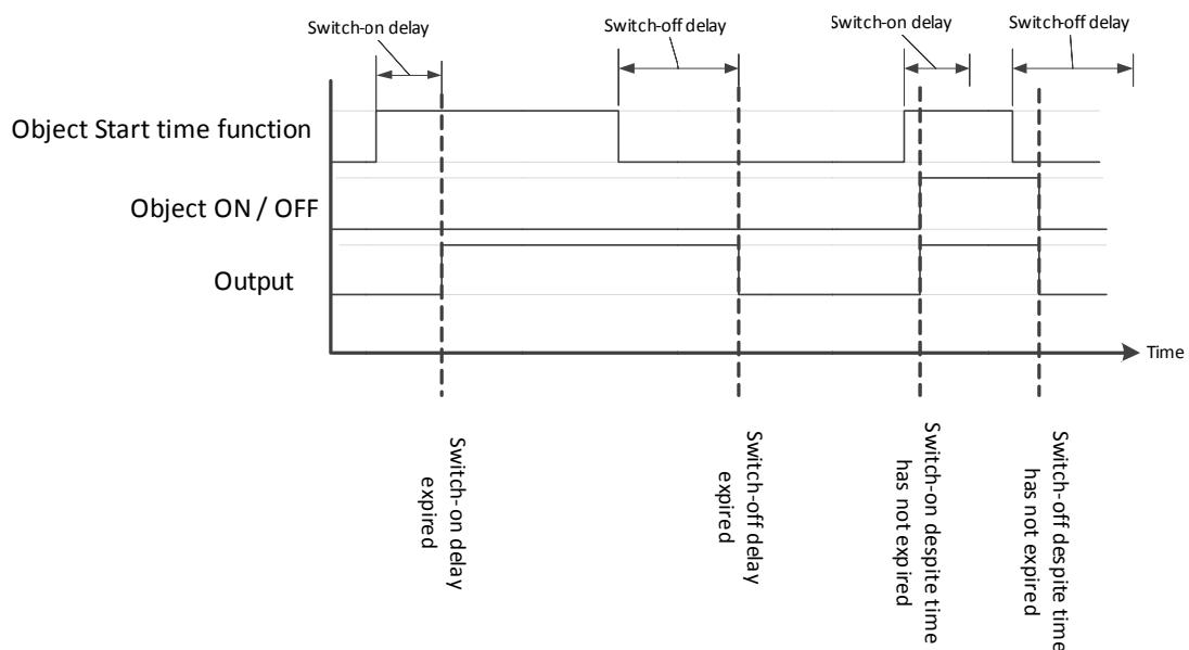
Messages for the object ON / OFF and changes on status via other functions have priority over ON- / OFF delay. If during a running ON – delay an OFF message will be received the delay will be stopped and the output stays OFF. If during a running OFF – delay an ON message will be received the delay will be stopped and the output stays ON.
