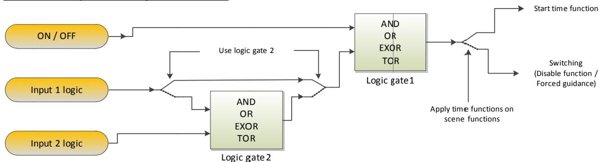
State transition diagram for AND, OR and EXOR linking's:
