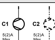
1-stage compressor and electric heater
