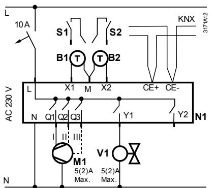
2-pipe / heating or cooling – ON/OFF
