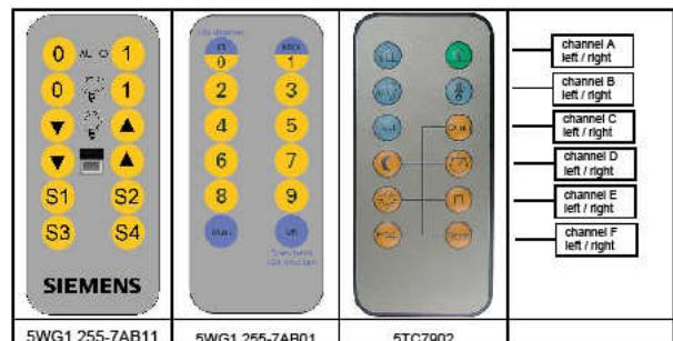
The IR decoder cannot distinguish between remote controls. The functionality of button pairs A to F (see above diagram) will be configured via the ETS.
