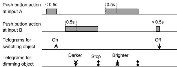
Function of input A/B: Dimming with cyclical sending, On/Off
