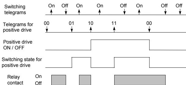
**9. Switching with OR function and time switch function, without positive drive**
