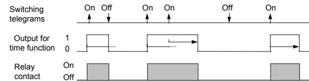
**6. Switching with AND function, without time delays or positive drive**
