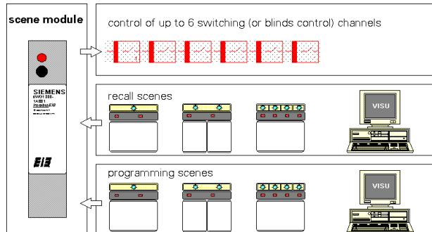
By employing more than one scene module any number of switching channels can be allocated to a single scene. However, no more than six scene modules (= 36 switching channels) should be accessed by a scene simultaneously. Otherwise hardly any information could be sent while the bus is busy dealing with the individual switching channels.
