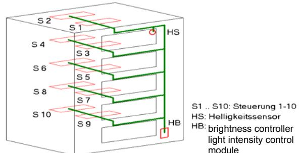
The brightness controller GE 253 measures the outside light intensity (the sensor points outside the window). Therefore the brightness controller must be protected from the artificial lighting to avoid any feedback. As the lighting conditions are almost identical all over the building front, one brightness controller is enough to generate the light intensity value to controlling all lights to that front of the building.
