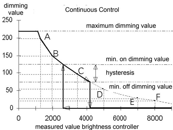
Changing the parameter "Response to min. dimming value" to "do not switch off" results in the below characteristic:
