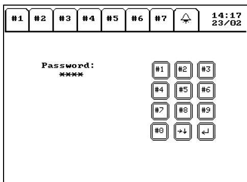
A 4-digit password must now be entered via the keypad. The password is defined in the ETS parameter settings. Once you have entered the password, the entry page for the time tasks appears.
