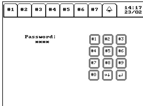
A 4-digit password must now be entered via the keypad. The password is defined in the ETS parameter settings. Agree this with your installer. Once you have entered the password, the entry page for the time tasks appears:
