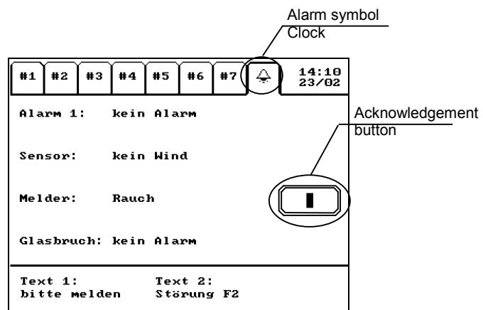
When an alarm occurs (object value 1 at object no. 214 to 217), the display automatically changes to the alarm page, the alarm symbol (clock) flashes and the alarm is clarified acoustically by a signal tone (adjustable). In addition, an acknowledgement button is shown on the right-hand side of the display.
