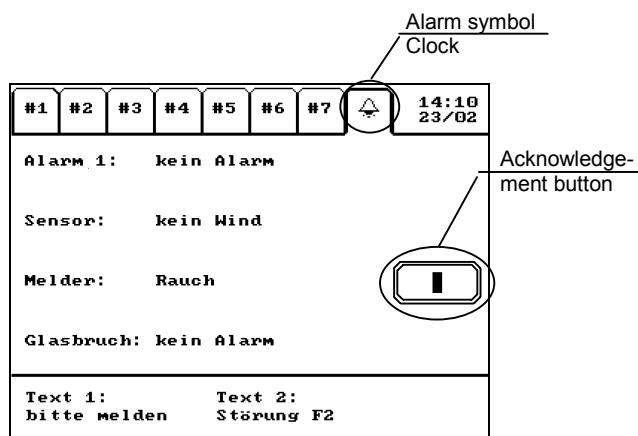
When an alarm occurs (object value 1 at object no. 214 to 217), the display automatically changes to the alarm page, the alarm symbol (clock) flashes and the alarm is clarified acoustically for an adjustable period by a signal tone. In addition, an acknowledgement button is shown on the right-hand side of the display.
