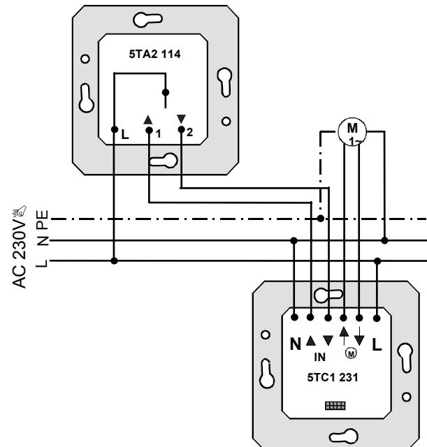
If the shutter pushbutton (5TA2 114) is used, the shutter can be controlled manually (UP/DOWN or STEP command) to move it to the desired position. An unlimited number of conventional extension units can be connected.
