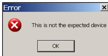
If the configured device type does not match that of the learned-in wave device, one of this error messages appears.
