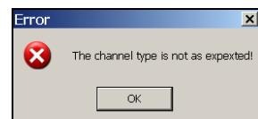
In the case of adjustable sensor channels, it is necessary to ensure that the parameterized sensor function (Switching, Switching/Dimming, Shutter, Scene) matches the function set at the wave device during learn-in. If this is not the case, this error message appears.
