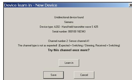
In the "Device learn-in" window, information is displayed on the various channel types (e.g. Configured channel type: Switching/Dimming. Learned-in channel type: Switching).
