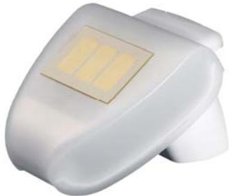
The AP 257/21 weather station (see figure 1) contains all sensors, electronic systems for weather data analysis and bus interfacing in one compact enclosure. It measures wind speed, brightness and temperature, detects dust / dawn and precipitation and receives the DCF77 radio signal for date and time.
