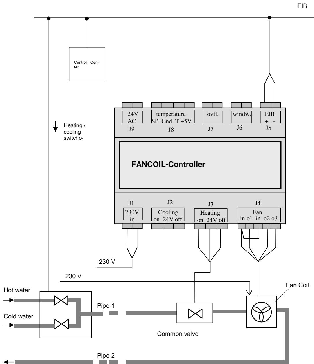
Hot water / cold water switching over is performed via a control center
