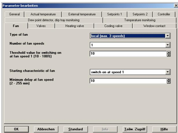
Choose “local” type of fan. Under “Starting characteristic”, however, “Switch on at speed 1” or “Switch directly on” should be selected.
