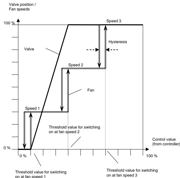
The valve opens on activation of fan speed 1 and opens up to a maximum of 100% at the end of speed 1.
