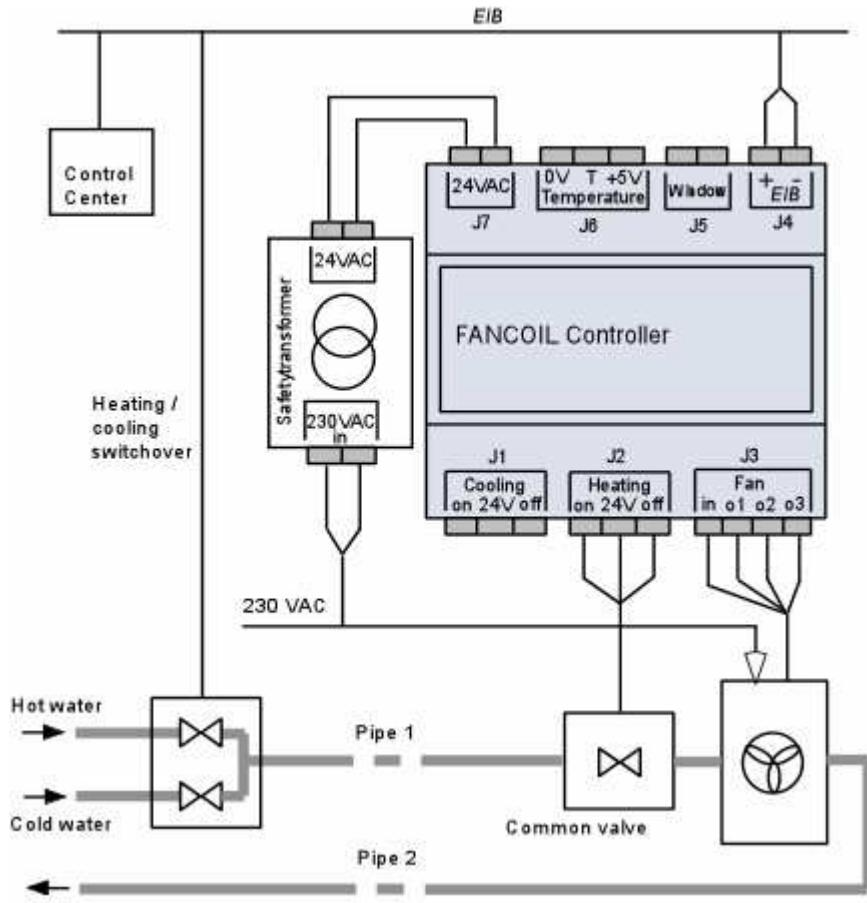
Hot water / cold water switching over is performed via a control center
