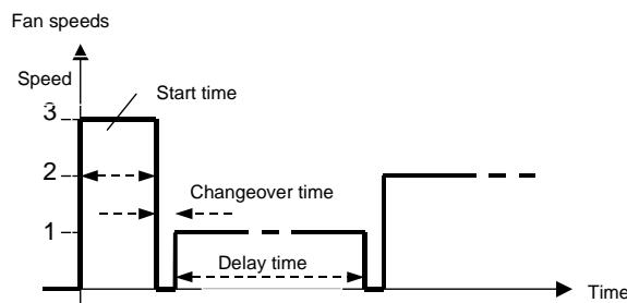
In this example, speed 3 was selected as the starting speed of the fan. The required speed is set following a start time and a changeover delay e.g. speed 1.
