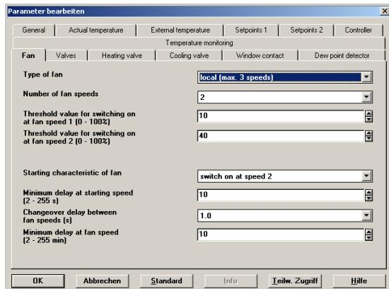
Choose "local" type of fan. Under "Starting characteristic", however, "Switch on at speed 2" or "Switch directly on" should be selected.
