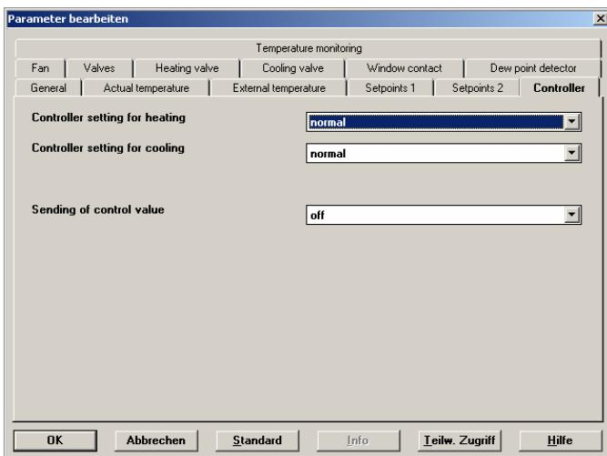
If one of the parameters is set to "user-defined", "controller setting for heating" or "Controller setting for cooling", further parameters become visible. Extensive knowledge of control technology in building automation is however necessary to carry out the correct settings.
