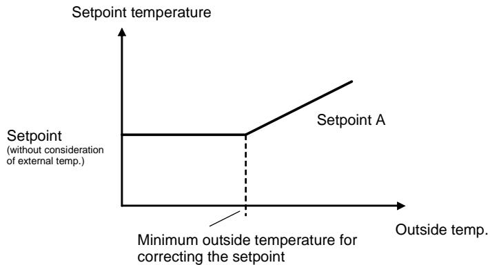
If the outside temperature is higher than the setting for **“Minimum external temperature for correcting the setpoint”** under **“Setpoints 1”**, the setpoint for cooling (Setpoint A) is calculated as follows:
