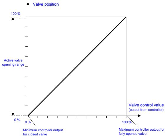
Diagram: no valve adjustment,
