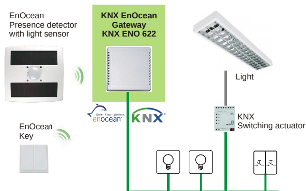
Fig. 7: Application example: light controller
