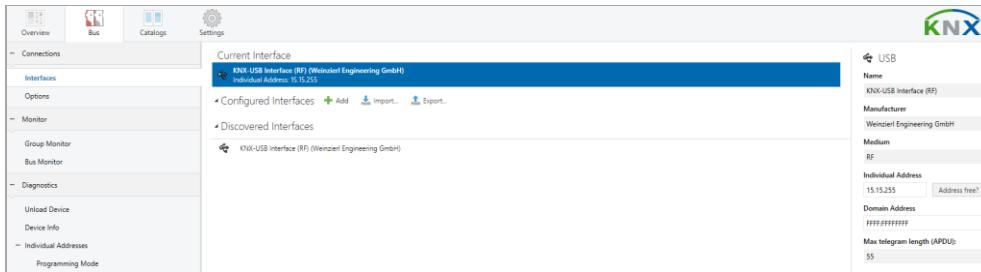
In the “Individual Address” section, the currently used individual KNX address can be changed. To check if the desired individual address is not already available in your KNX installation, the button “Address free?” can be pressed.
