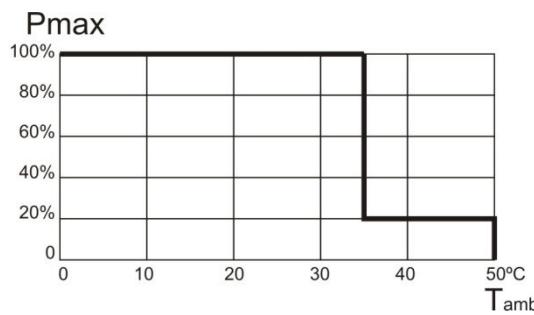
**Note II:** *When the Ambient Temperature is high, the Dimmer adjusts itself to the 20% brightness (according to the diagram), avoiding any problem arisen from an excessive over heating that could be harmful for the electronic of the device.*
