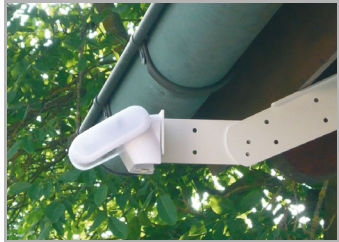
Fig. 8 Example use of the hinge arm mounting: With the hinge arm mounting, the weather station projects from beneath the roof overhang. Sun, wind and precipitation can act upon the sensors without hindrance.
