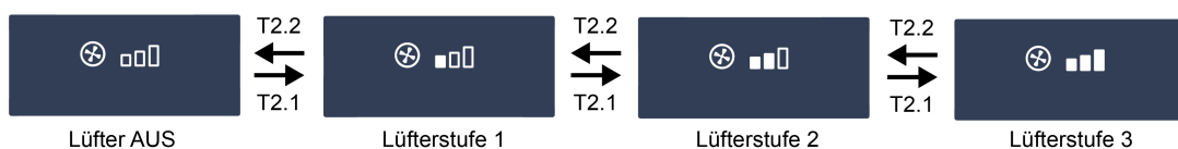
Image 8: Setting of manual fan control (operating level)
