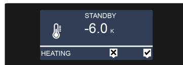
Image 27: Increasing the heating setpoint temperature (menu level 2)
