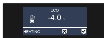
Image 23: Increasing the heating setpoint temperature (menu level 2)
