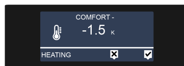
Image 19: Increasing the heating setpoint temperature (menu level 2)
