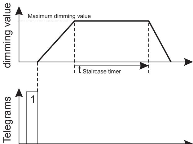
You can activate the staircase lighting function for a channel via a parameter:
