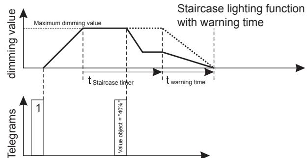
If you have parameterised a cut-out delay for the dimmer output, the warning time will begin after the delay period has expired.
