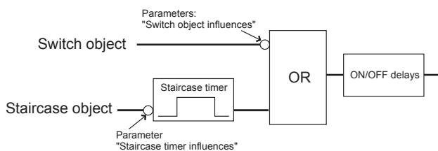
You can invert, or not invert, the effect of the two object values on this logic operation using parameters:
