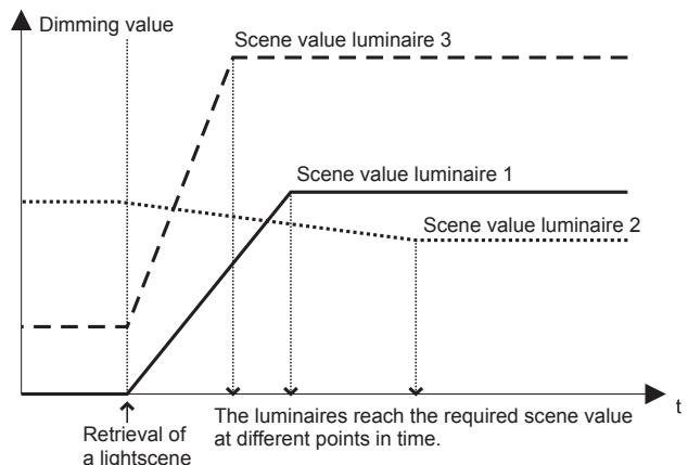
The "Same dimming time" function can be used to synchronise the different dimming times of the channels in such a way that all channels reach their setpoint value at the same time. Using the "Time factor modifiable via the bus" parameter (via the communication object "Factor same dimming time"), the dimming times can also be synchronised for several dimming actuators.
