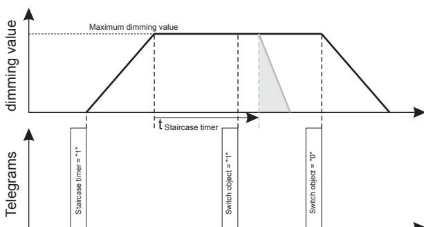
The brightness of the logic operation result and the dimming speed is defined by the last telegram (see the charts below).
