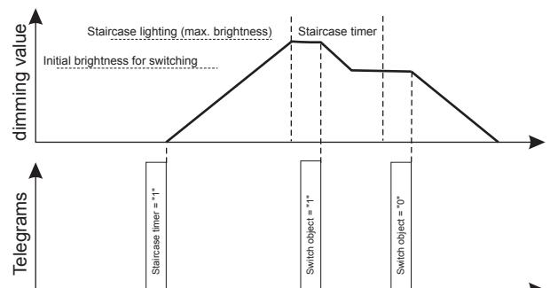
You can use this, for example, for temporary continuous light switching (cleaning lighting). An ON telegram from the switch object causes the light in the staircase lighting function to remain switched on continuously. Value, dimming, scene and central telegrams continue to be effective, however. For an application of this type, an initial brightness of 100% would be useful.
