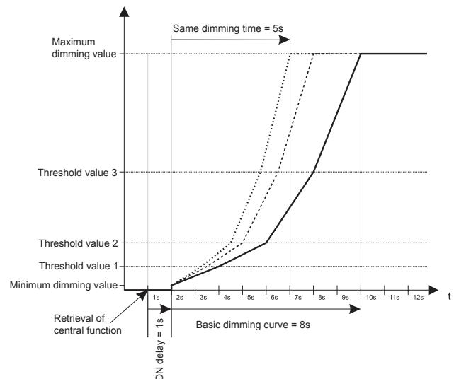
The ON delay is also retained even with a "same dimming time". The dimming curve is compressed or extended in such a way that the dimming value is reached after the same dimming time. In other words, calculation of the new dimming curve takes into account the pure dimming time (the same dimming time minus ON delay time).
