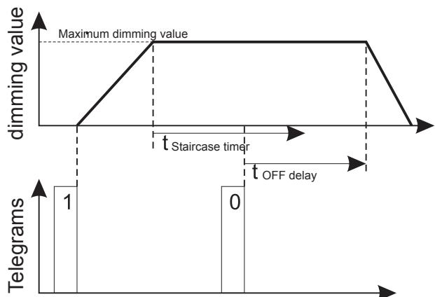
If you have selected the parameter value "without manual OFF", the staircase lighting function will not be interrupted when a telegram with the value "0" is received, but will continue to run normally until the staircase timer has expired.
