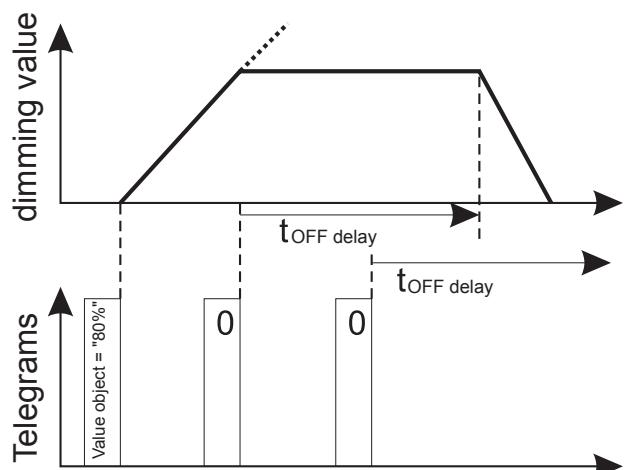
If the output receives a new telegram while an OFF delay is active, which creates an ON status, the OFF procedure will be halted and the new setpoint value set.
