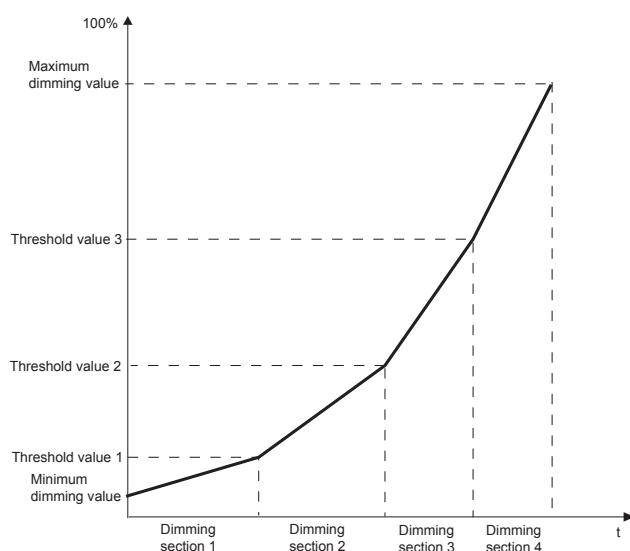
**i** Note: The dimming curve (the actual voltage curve applied to the output over the time period) is still influenced by the dimming time reductions of the dimming reduction sets and the dimming time reduction object; refer to the section on dimming speed.
