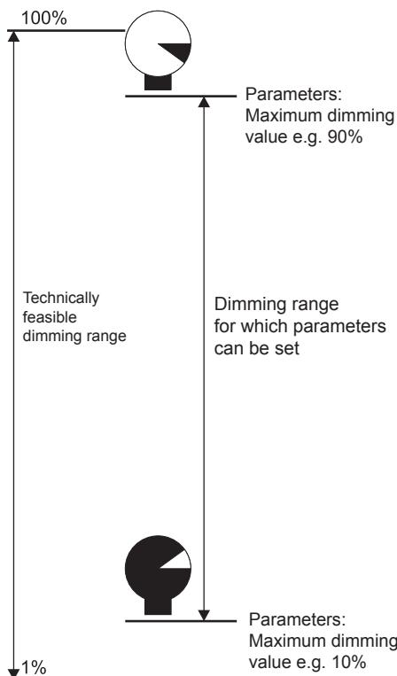
The parameterisable dimming range is set using the following parameters:
