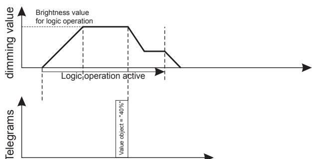
The brightness of the logic operation result and the dimming speed are defined by the last telegram.
