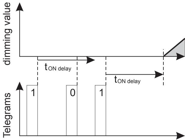
You can use a parameter to set whether the output channel remains switched off during the ON delay, or whether it is already set to the minimum dimming value.
