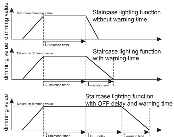
Regardless of which dimming value the output has after the staircase lighting function has expired, the time duration for the dimming-down procedure always corresponds to the warning time when the cut-out warning is active.
