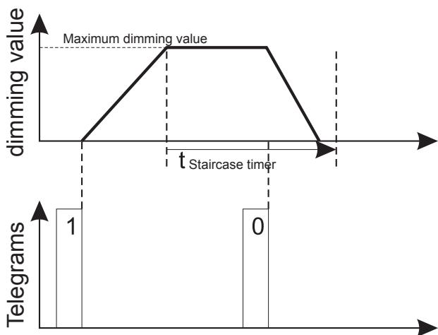
If an OFF delay has been parameterised, this function will now be active and the output will only switch off after the delay time has expired.
