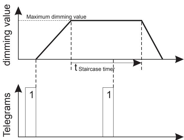
..., retriggerable: If the "Staircase lighting" object receives an additional "1" telegram while a staircase lighting function is active, the staircase timer will be restarted. This occurs when a "1" telegram is received while the function is active.
