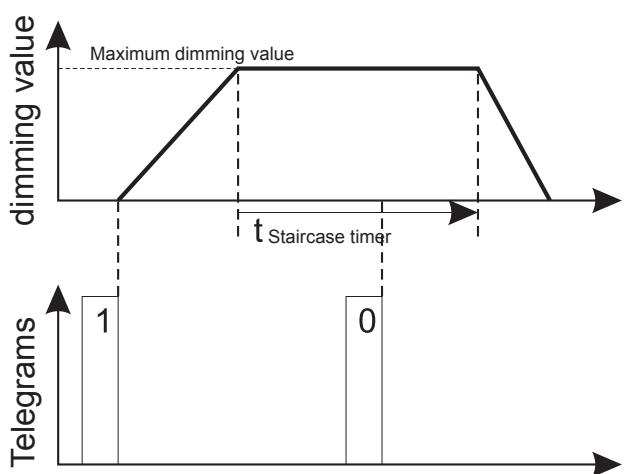
..., not retriggerable: With this setting, the staircase lighting function which was started initially proceeds normally, even when additional "1" telegrams are received during the staircase timer.
