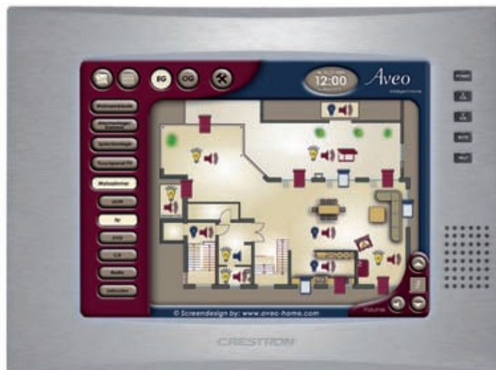
Crestron wall-mounted touch-panel with video display
