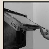
[ Mounting support for comfortable mounting and connecting ]
